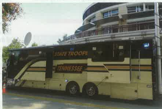
A popular display was the Tennessee Highway Patrol's Mobile Inspection Station – the only one of its kind. The $1.4 million MIS bristles with technology, including a dispatch/communication system, satellite communication, infrared camera and a 360-degree rotating elevated camera. The station can also serve as an emergency command post.
